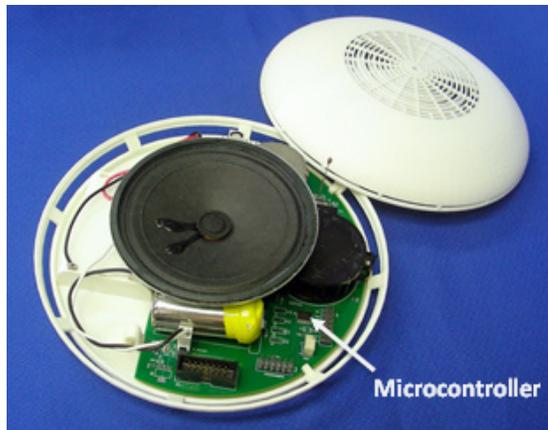
Figure 4. Assembled prototype incorporating multiple sensors, a microcontroller, power (three AA batteries), and a speaker for 520 hertz alerting. The enclosure is 6.5 inches in diameter and 1.7 inches tall.
